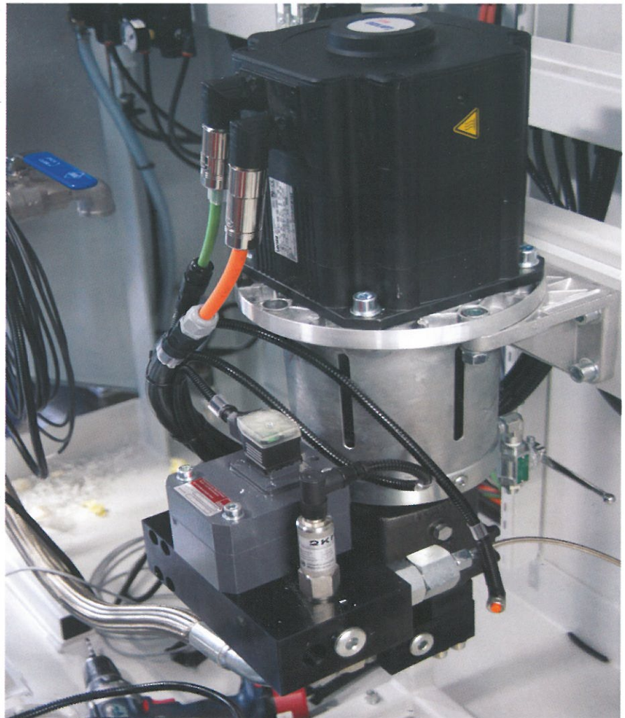
Servo Driven Metering pump with Flowmeter for feedback.
