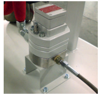
Volume counter for metering control
