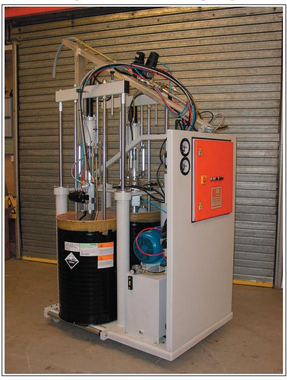
Piston Metering System for High Viscosity Materials
